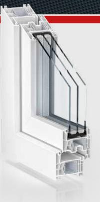
KBE 76 makes it easier and more convenient than ever before to achieve energy and heating cost savings. The new generation of windows can incorporate triple glazing and functional glazing up to a thickness of 48 mm. In other words: hardly any heating energy is lost through the glass. Yet the expansive glass surfaces allow valuable sunlight warmth to enter.
