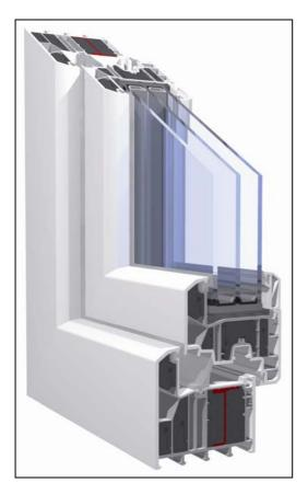
With its variant featuring a rebate base bonding, the "System\_88mm PAS-SIVHAUS" exhibits a  $U_f$  value of 0.79 W/(m<sup>2</sup>K), representing the expansion stage with the maximum thermal insulation in the 88 mm KBE profile series.
